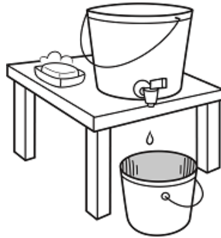
A bucket with a tap for handwashing. Used wash water is collected in a bucket below and disposed of in a garden or soak pit.
