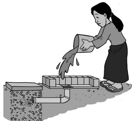
Disposing of used wash water in a soak pit
