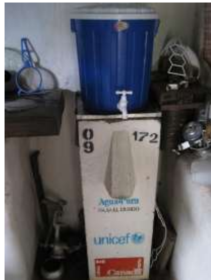
APPM Concrete BSF, Honduras
