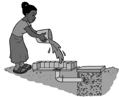
Disposing wastewater in a soak pit
