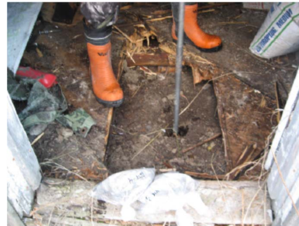
Photo 2: Photo of hand-augered borehole BH108 extended beneath abandoned building.
