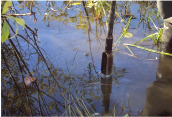
Photo 2 – View of hydrocarbon sheen in Eabamet Lake while collecting sediment sample A-SED1.
