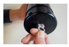
7. Insert the battery compartment into the casing and place the supplied tool into the screw on the bottom of the receiver to turn clockwise until the gap by the main O-rings is completely closed. Do not tighten with force.
