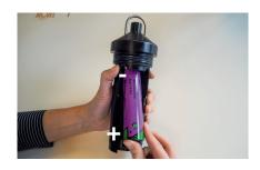
3. Insert the battery with the minus towards the spring. Ensure that the battery spring is compressed correctly while sliding the battery in and clicking it into place.
