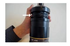
6. Check O-rings for deformation and cracks. An initial sealing force is needed, must be round and not square. Only use light lubrication with silicon or O-ring grease for ease of installation. Sealing surfaces free of scoring and scratches.
