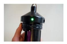
4. The LED indicator will flash yellow during start-up. These flashes show the boot sequence and self-checks. When complete, the LED indicator will flash 3x3 green right andthe receiver starts listening for acoustic signals.
