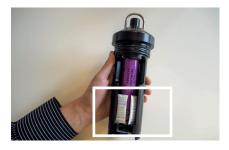
5. Put two humidity-absorbent bags in the opening over the battery. Check the colour of the pellets for quality. Blue color pellets are ready to deploy, white/translucent needs to be dried or replaced.
