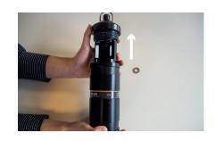
2. Pull the battery compartment and receiver top to seperate from the casing.
