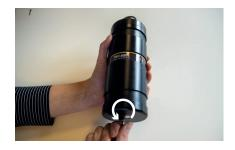
1. Open the housing using the supplied tool (or a coin, screwdriver, power drill etc.) and turn counterclockwise to expose the battery compartment.
