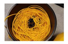
4. Carefully flake the rope into the RopeBox. Do not pre coil or tightly twist the rope around the centre stem. This may cause knots et release.
