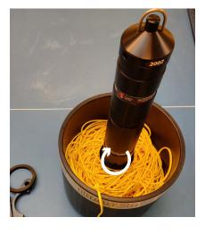
8. Carefully place the receiver over the centre stem and turn the receiver clockwise until fully engaged on the threads. Ensure that the receiver is fully attached by checking that there is no gap between the bottom of the receiver and the central stem. If there is too much resistance, the motor may turn and you need to unscrew and inspect the threads again. The centre stem must be replaced if the threads are damaged.
