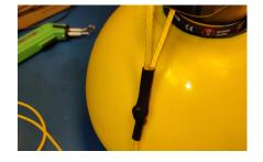
15. Put an adhesive lined heat shrink on the rope, before tying the rope to the collar with a secure knot (e.g. bowline or double figure eight). Lightly apply heat gun to the heat shrink. Do not melt the rope.
