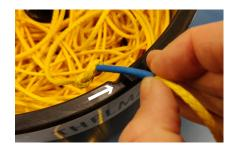
12. Ensure the rope exits in the machined grove at the edge of the RopeBox.
