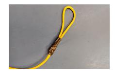
16. Apply a similar loop knot and heat shrink operation as above to the mooring end of the rope.
