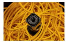
6. Inspect the o-ring on top of the RopeBox centre stem for damages or debris, and lightly lubricate it. Inspect the internal threads damage and debris.
