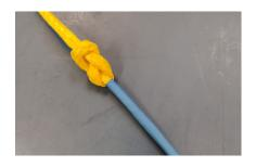
2. Measure the required length of free rope for mooring attachment and tie a figure eight stopping knot to the rope. For extra security/protection, put a piece of heat shrink below the knot to avoid chafing. Lightly apply heat gun to the heat shrink. Do not melt the rope.
