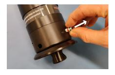
7. Remove the Key Pin and the short Release Lug if present in the receiver casing.
