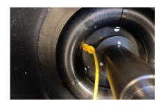
3. Pull the free end of the rope through from the inside of the box, through the hole in the bottom. Ensure that the stopping knot does not pull through the hole.
