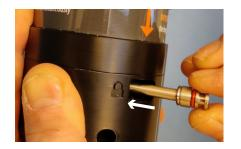
9. **IMPORTANT**: Insert the key pin back into the **LOCKED** deployment position. You may have to turn the release lug slightly counter clockwise to align key pin with the release lug flats. Make sure the Key Pin clicks securely into place.
