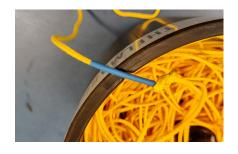
5. Place a stopping knot and heat shrink above the knot approximately 50 cm from the top end of the rope. Lightly apply heat gun to the heat shrink. Do not melt the rope. Leave this end of the rope on the outside of the RopeBox.
