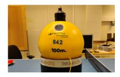
11. Slide the buoy over the receiver.
