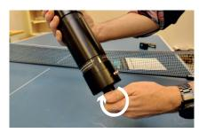
9. Insert the receiver into the casing and turn the release lug clockwise until the gap by the main o-rings is completely closed. Do not tighten with force.
