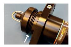
7. Check O-rings for deformation and cracks. An initial sealing force is needed, must be round and not square. Only use light lubrication with silicon or O-ring grease for ease of installation. Sealing surfaces free of scoring and scratches.
