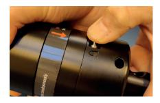
10. IMPORTANT: Remove and re-insert the Key Pin back into the **LOCKED** deployment position. You may have to turn the release lug slightly counter clockwise to align key pin with the release lug flats. Make sure the Key Pin clicks securely into place. A piece of electrical tape can be applied over the holes to prevent marine growth in the Key Pin mechanism.
