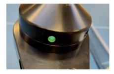
5. The LED indicator will flash yellow a few times during start-up. When the boot sequence and self-check complete, the LED indicator will flash 3x3 green right before the receiver starts listening for signals.
