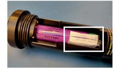
6. Put two humidity absorbent bags in the opening over the battery. Check the colour of the pellets for quality. Blue colour pellets are ready to deploy, white/translucent needs to be dried or replaced.
