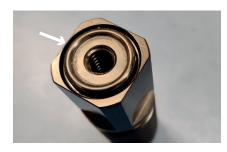
8. Remove the Key Pin from the unlocked service position and remove the release lug. Lightly lubricate the o-ring. Reinsert the release lug and the key pin into unlocked service position.
