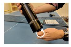
3. Turn the release lug counter clockwise to open and expose the battery compartment.
