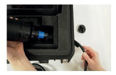
11. Unscrew the dust cap from the connector of the 5m Live Ecomate cable, remove the small lid on the right side of the DeckBox field case, slide the cable through and attach the 5m Live Ecomate cable to the Link BT. Keep the lid in the case.
