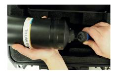
**16.** The power switch of the unit is located inside of the Ecomate connector. Remember to disconnect cable from Link BT after use. The battery is completely disconnected once the cable is separated from the Link BT.
