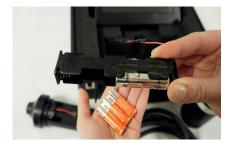
7. The battery holder has four slots for AA batteries. One of them is pre-loaded with a dummy battery to match the total voltage correctly.
