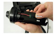
**9.** Connect the battery leads into the pictured connector on the outside of the compartment and slide the metal disc back into place.
