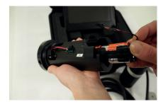
**8.** Insert the battery holder back into its compartment.
