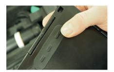
**13.** Locate the Surface Go tablet and make sure it is charged. Turn on Surface Go tablet (long, hard push of the button on the backside of rugged casing).
