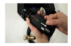
**6.** Remove the metal disc and release battery leads to expose the battery compartment.
