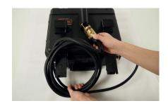
**2.** Release the Live with cable from its holder on the lid of the field case.
