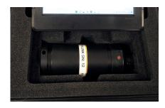
**12.** The LED indicator will flash 3 x green immediately when connected, followed by a yellow flash when the Link BT has detected the Live. The LED indicator will then flash red two times every five seconds until LiveView connection is established.
