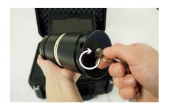
**10.** Close Link BT main unit. Screw clockwise only until the gap by the top closes. No extra tightening is needed to seal.
