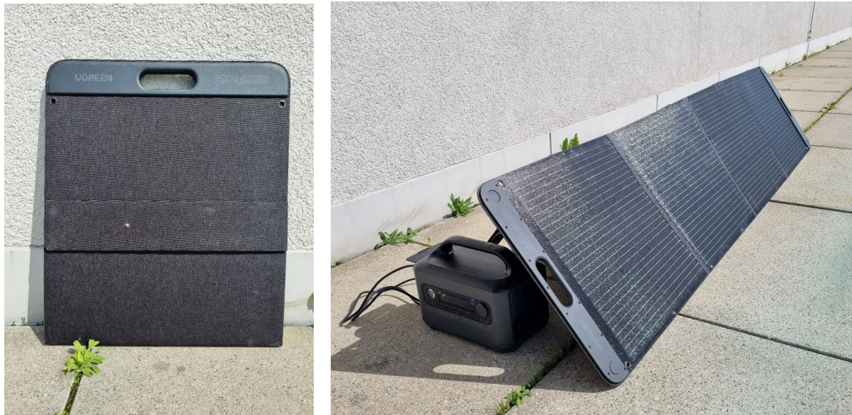
Figure 20 Solar bag (200W) with storage (680Wh)
