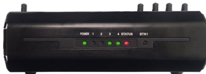
Figure 4-1: Front panel LED indicators — all LEDs green indicates normal operation with active RF channels.
